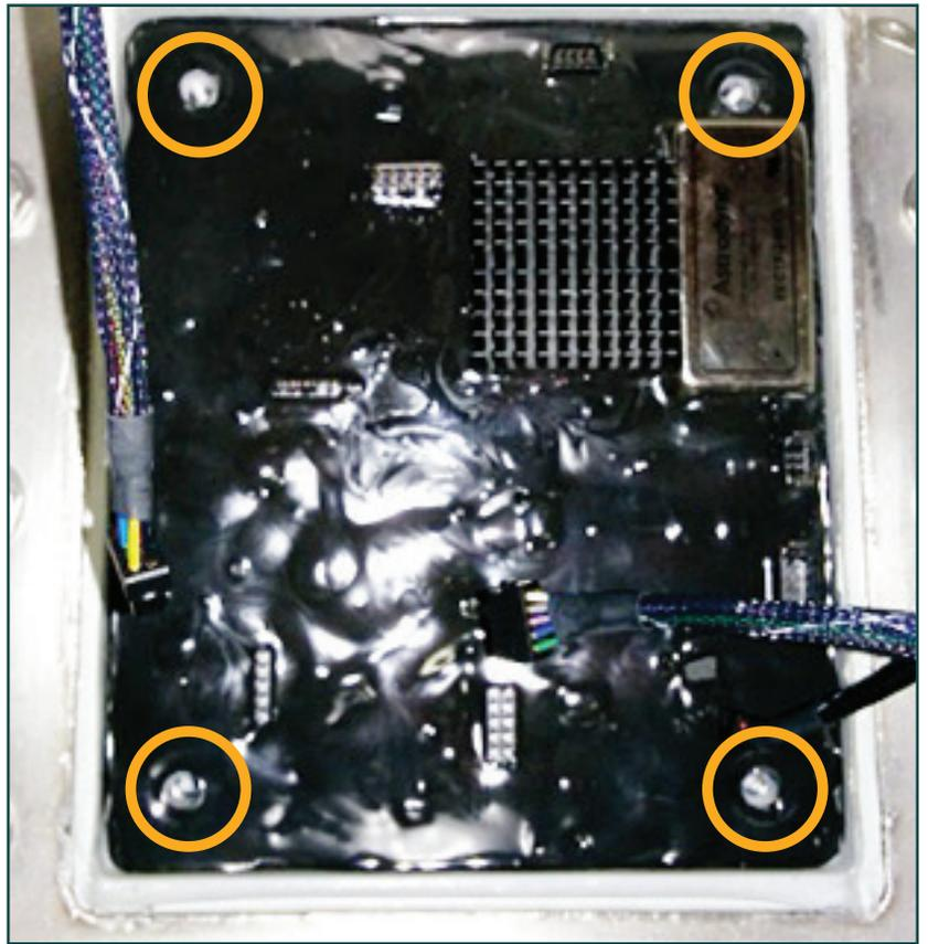
8: Remove screws securing the Circuit board
