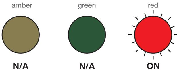
Unit is sensing an Error
